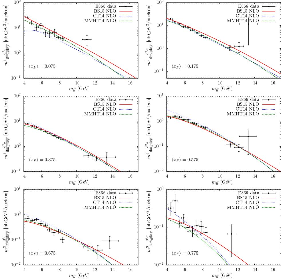
Figure 7: The DY differential cross section measured in the di-muon channel by the E866 Collaboration at  $\sqrt{s} = 38.8$  GeV [20] over a low-mass range and various Feynman  $\langle x_F \rangle$  variables vs QCD NLO predictions obtained by using PDF models from Refs. [3, 4, 5].
