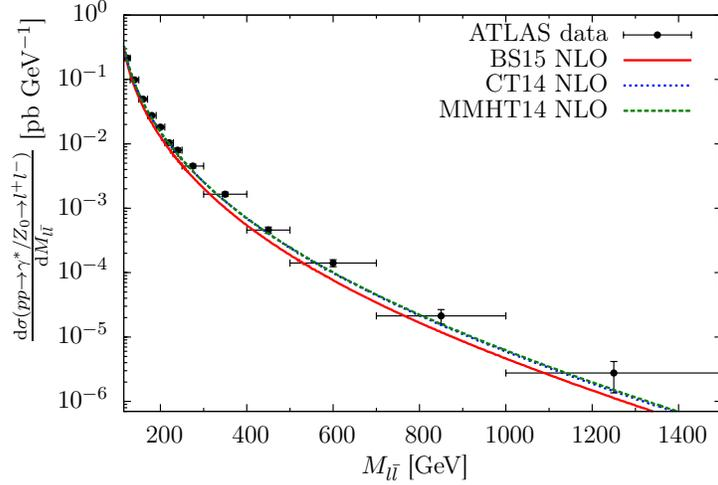
Figure 6: The DY differential cross section measured in the di-electron channel by ATLAS at  $\sqrt{s} = 7$  TeV over the high-mass range 116 – 1500 GeV [18] vs QCD NLO predictions obtained by using PDF models from Refs. [3, 4, 5].
