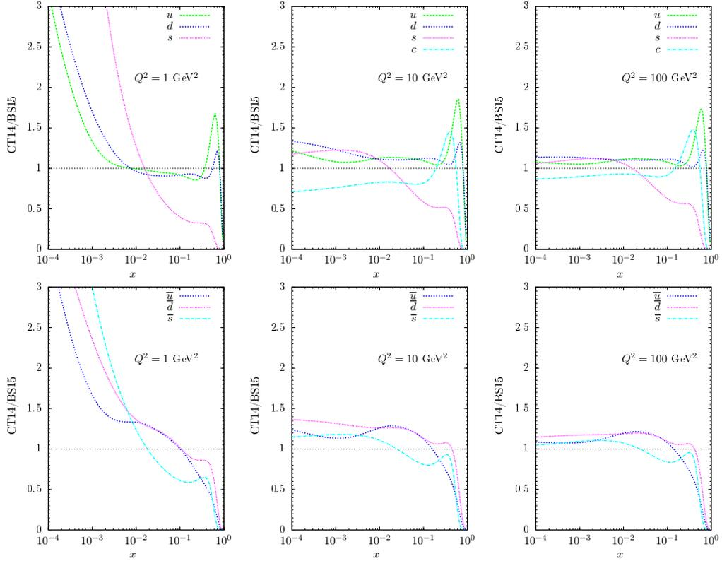
Figure 13: The CT14-to-BS15 ratios for quark (upper row) and antiquark (lower row) NLO PDFs as functions of  $x$  and  $Q^2 = 1, 10, 100$  GeV<sup>2</sup>.
