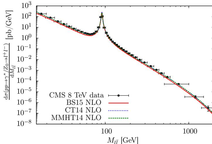
Figure 4: The DY differential cross section measured in the combined di-muon and di-electron channels by CMS at  $\sqrt{s} = 8$  TeV over the invariant mass range from 15 GeV to 2 TeV [13] vs QCD NLO predictions obtained by using PDF models from Refs. [3, 4, 5].
